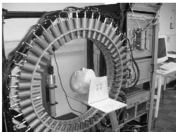
Fig. 1. The PET detector array and supporting equipment. The VME crate to the right handles all signal processing.
